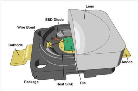
**Figure 1: Internal construction of the Diamond DRAGON<sup>®</sup>**
