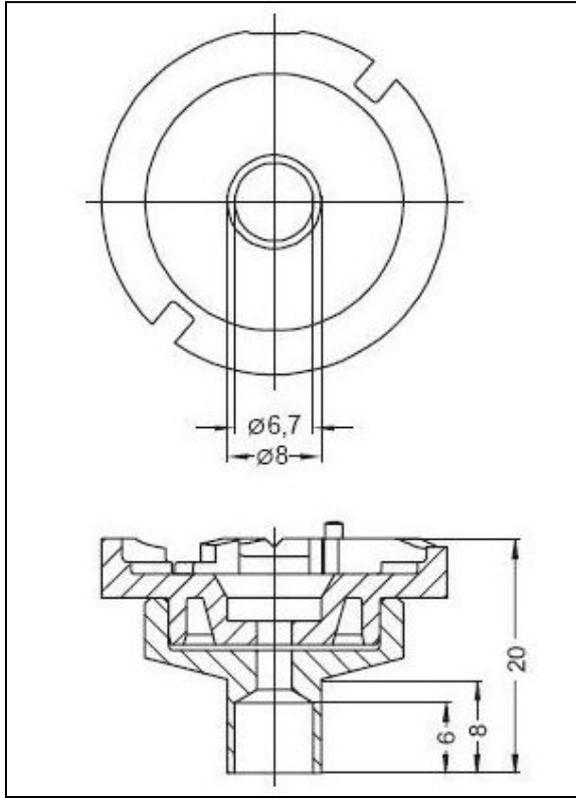
**Figure 5: Recommended design for the pick & place tool of the Diamond DRAGON®**
