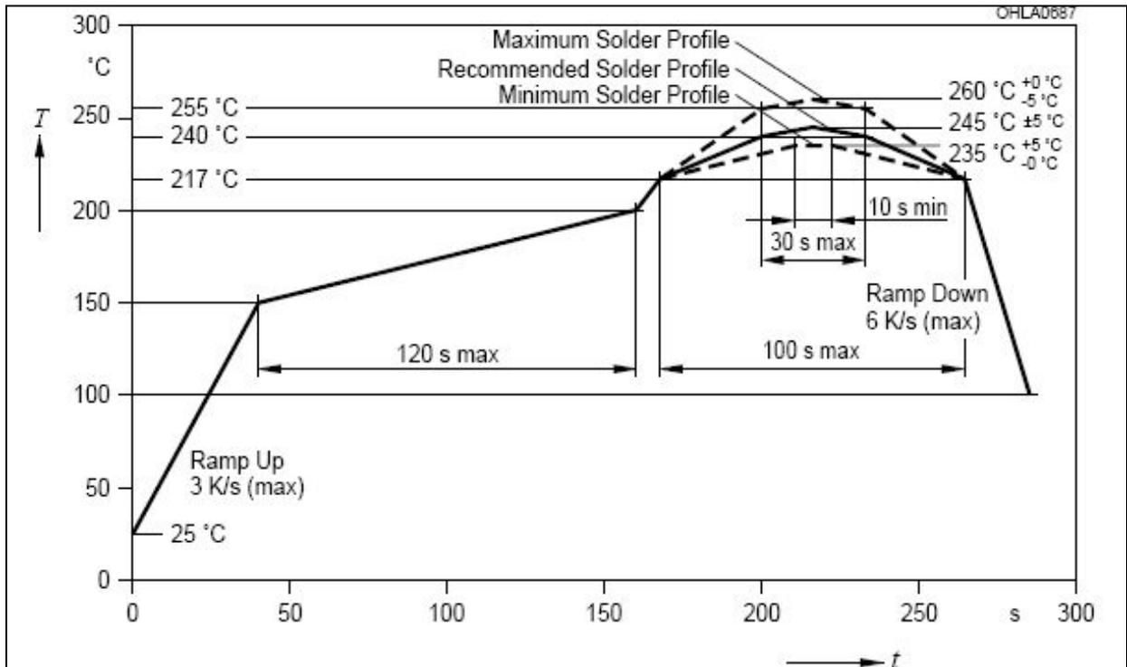
Figure 6: Reflow solder profile for lead-free soldering of the Diamond DRAGON®
