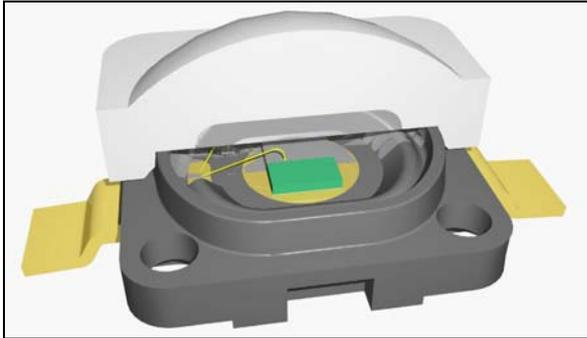
**Figure 3: Cross section through Diamond DRAGON®, mounting of the lens over the functional area**
