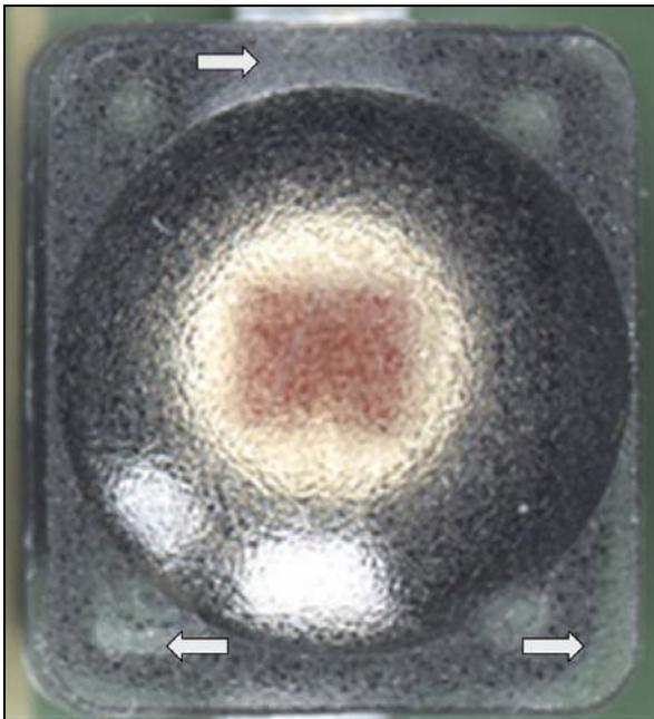
**Figure 4: Selective gaps in contact adhesion between the boundary of the lens and housing after soldering**
