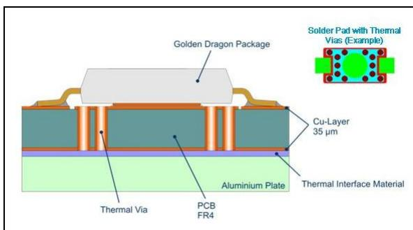
**Figure 8: Conceptual layout of FR4 with thermal vias**
