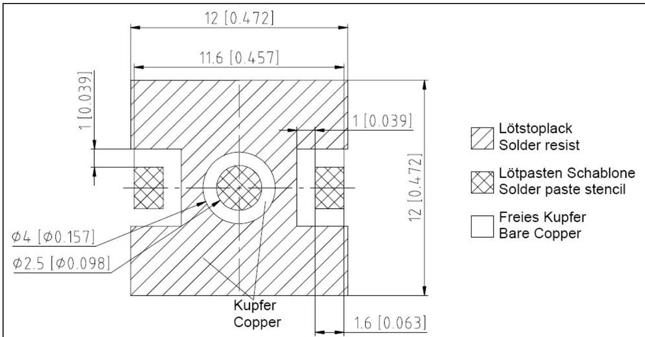
Figure 7: Recommended solder pad for the Diamond DRAGON®
