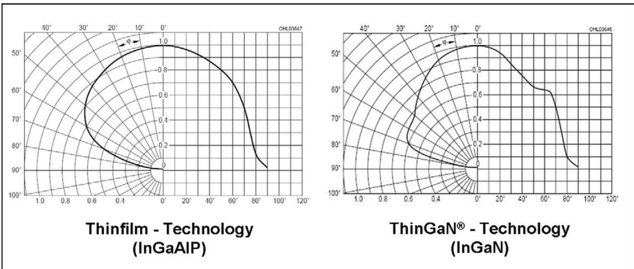
**Figure 2: Radiation characteristics of the Diamond DRAGON<sup>®</sup>**
