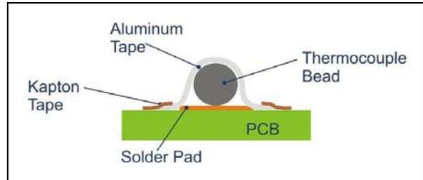
**Figure 5: Attachment with aluminum and polyimide tape**
