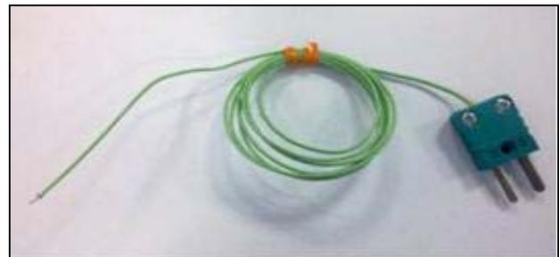
**Figure 1: Example of a type K thermocouple**
