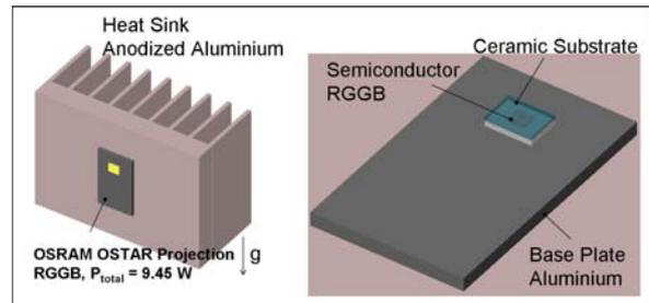
Figure 8: Construction of OSRAM OSTAR Projection with heat sink
