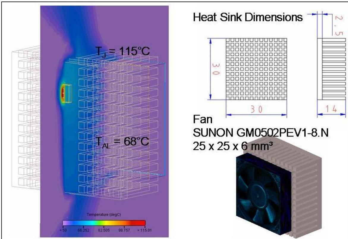
Figure 11: Simulation results of OSRAM OSTAR Projection with a minimized cooling element
