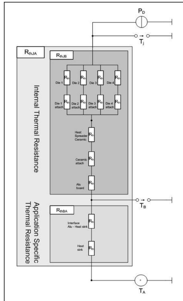
Figure 2: Static equivalent circuit
