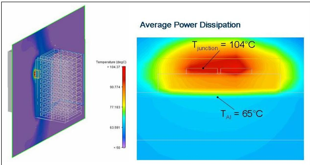
**Figure 12: Simulation results of OSRAM OSTAR Projection in pulse operation, average temperature level**
