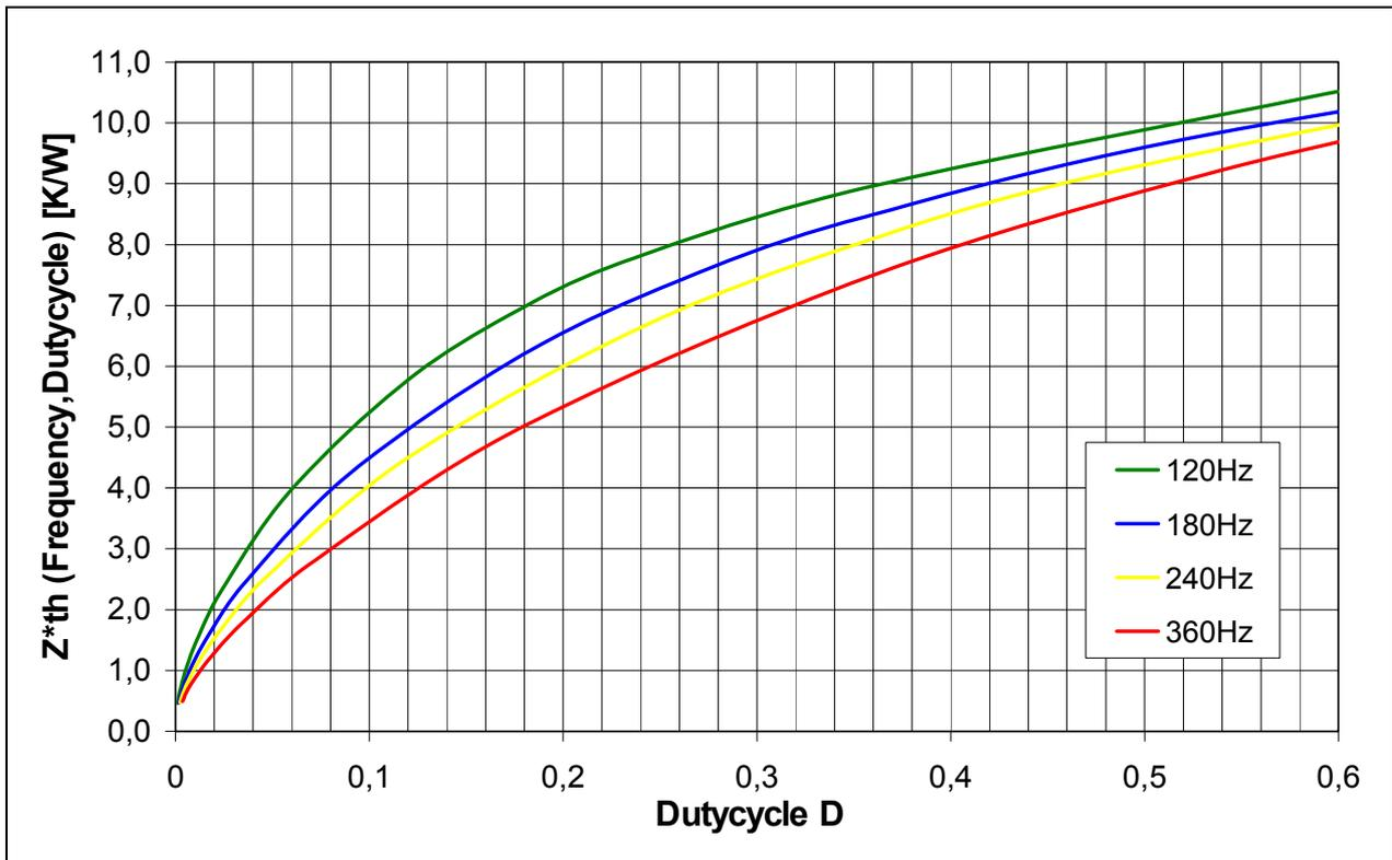
Figure 3: Thermal resistance for OSRAM OSTAR Projection module, pulsed operation of 1 chip
