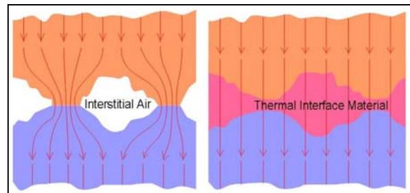
**Figure 14: Heat flow without/with thermal interface material**
