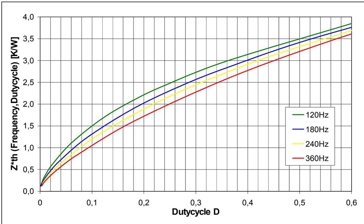
Figure 5: Thermal resistance for OSRAM OSTAR Projection module, pulsed operation of all 4 Chips
